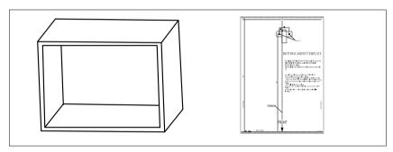
2. Make the marks on the bottom plane of cabinet according to marks "a" of the template.
