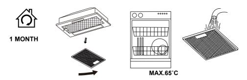
**Aluminium filters:** To avoid fires, clean thoroughly once a month or whenever the display pilot light lights up (if fitted). To do so, remove the filters and soak in hot water and detergent for an hour. If using a dishwasher, position the filters vertically to improve the cleaning process.
