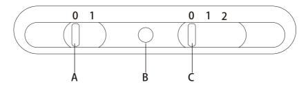
Motor control light(Ref. B) Light switch(Ref. A) 3 position motor control swtich(OFF, 1st and 2nd speed position) (Ref.C)
