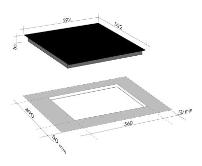
\*Note: The safety distance between the hotplate and the cupboard above the hotplate should be at least 760mm
