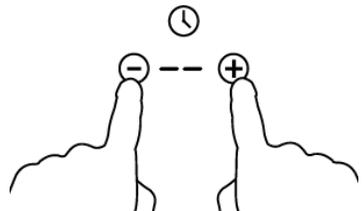
5. When the time is set, it will begin to count down immediately. The display will show the remaining time and the timer indicator will flash for 5 seconds.
