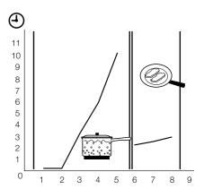
You can get a necessary heat setting in a shorter time if you activate the Automatic Heat Up function. This function sets the highest heat setting for some time (see the illustration above), and then decreases to the necessary heat setting.
