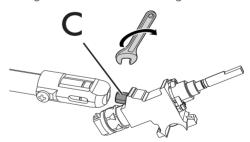
2. Use a spanner to remove the nozzles "C" and install the new ones for the required gas supply, following the indications given in the relevant table (see ""Burner and nozzle specifications table"").
