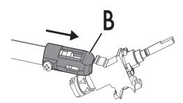
3. Reposition support "B" so that nozzle "C" is covered completely.
