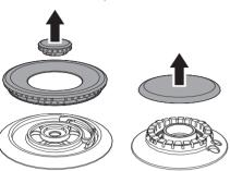
4. Unscrew the screws under each burner to remove the fixing plate.
