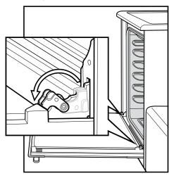
To then remove the top trim, press the ribbed release • clips at each end and lift top cap away from the door.
