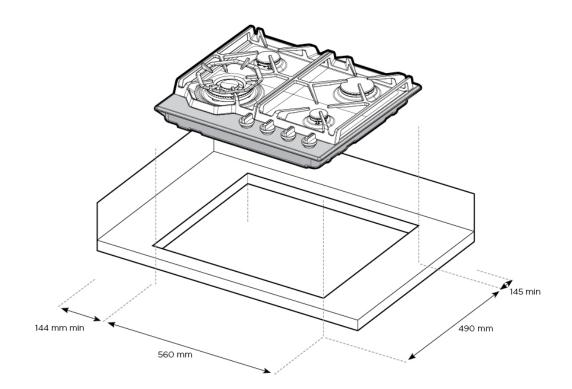
NOTE: Distances shown to adjacent walls/surfaces are for the distance to a combustible surface. If the surface is not combustible the measurement can be smaller than that shown.
