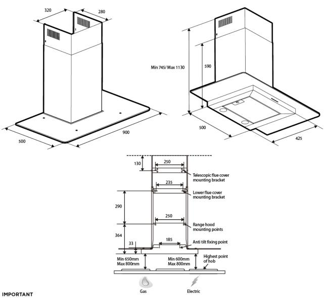
These dimensions are a guide only. All measurements are in millimetres (mm). For complete installation instructions, refer to the manual provided with product.
