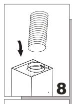
Connect the hose with the air duct.
