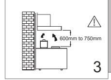
We recommend that after installation the bottom of the hood should be no less than 600mm and no more than 750mm above the stove's heating elements and burners.
