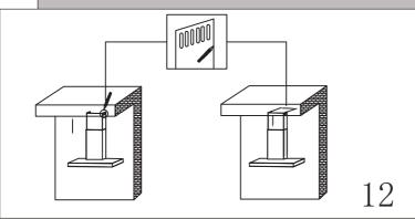
According to the dimension of the chimney fixed bolster, make sure the position of the two chimneys.
