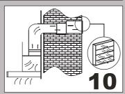
If your kitchen has a soffit above the cupboards, you may run the duct up into the soffit and then discharge horizontally through the outside wall to a wall cap.
