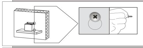
Screw down the four screws. first screw down the upper two screws, then screw down the others.
