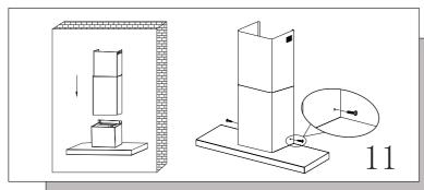
Put the outer chimney and inner chimney together on the windshield.
