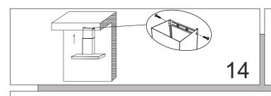
Use the Screw ST4\*10 to connect the chimney fixed bolster and the upper chimney.
