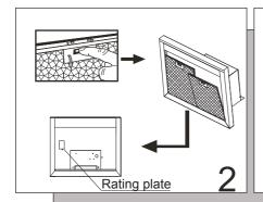
Check voltage and Frequency given on the rating plate located on the inside of the hood.
