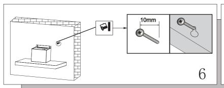
Hang the hood and let it's two installation holes aim at two screws, adjust it to setting position.
