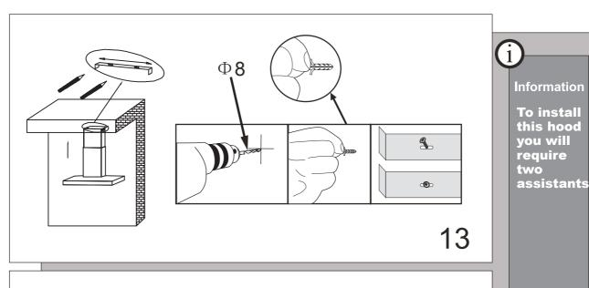
Install the chimney fixed bolster on the corresponding position on the wall.
