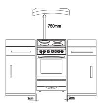
• The cooker should stand on a hard, even floor (do not put it on a base.)
