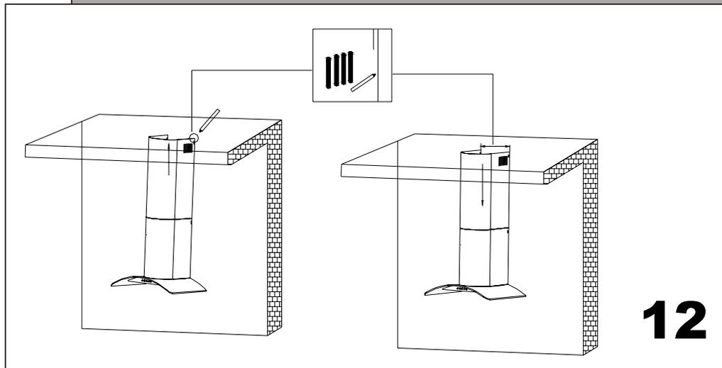
Measure the height for the chimney flue bracket. Pull the inner chimney to the desired height.
