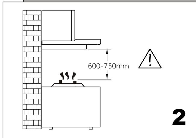
Ensure the hood is installed so that the bottom of the hood is no less than 600mm and no more than 750mm above the cooking elements or burners.
