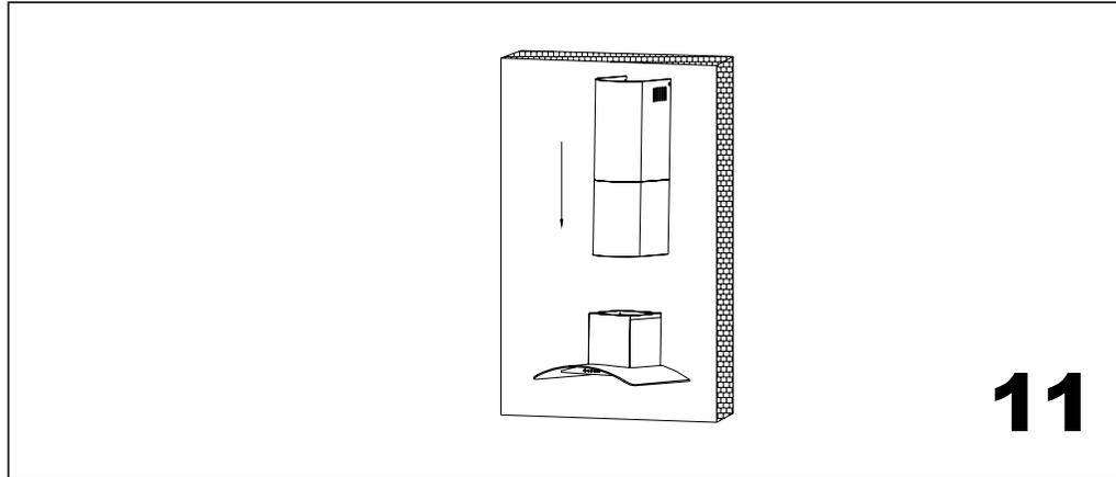
Assemble the 2 flues, inner top to outer bottom. Place them onto the hood body covering the air duct assembly and screw into place.
