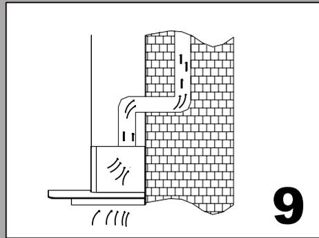
Vertical discharge of air. Run the ducting through a cupboard and/or into a space in the ceiling cavity to a roof cap.
