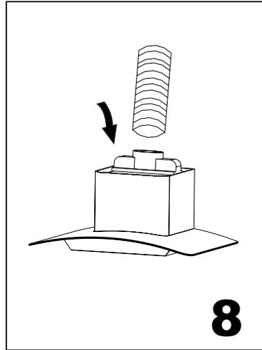
Attach the ducting hose to the air duct.
