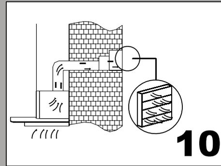
Horizontal discharge of air. Run the ducting through the eaves (soffit) and the outside wall to a wall cap.
