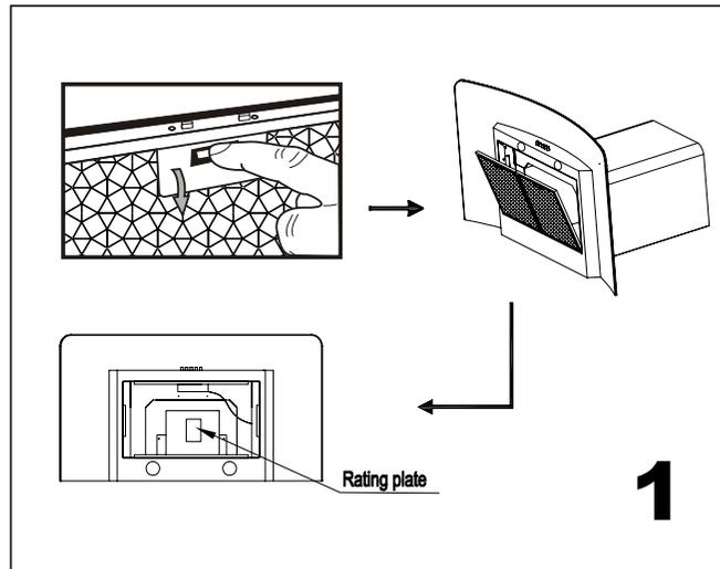
Check the voltage and frequency on the rating plate located inside the hood.
