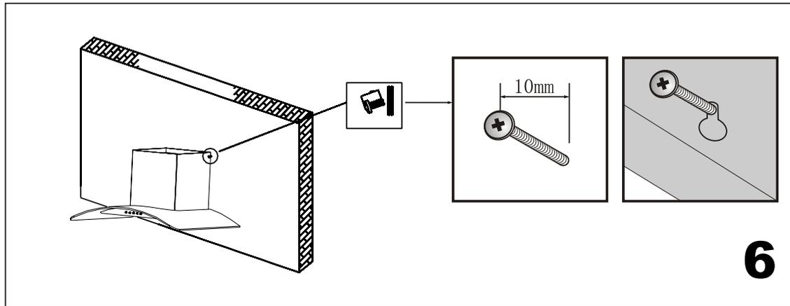
Hang the hood body onto the screws. First screw in the top 2 screws then the bottom 2 screws. Adjust the level of the hood on the wall to be straight horizontally.
