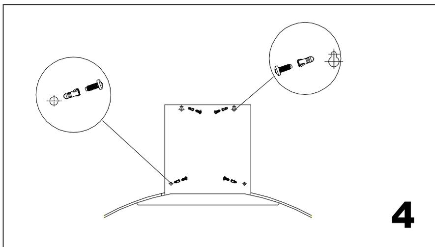
Using the drill hole stencil mark the screw positions on the wall. Drill four 8mm holes into the wall. Put one expansion plug and one 10mm screw into each of the holes. Screw the screws into place but not all the way into the plugs until after you hang and adjust the hood.
