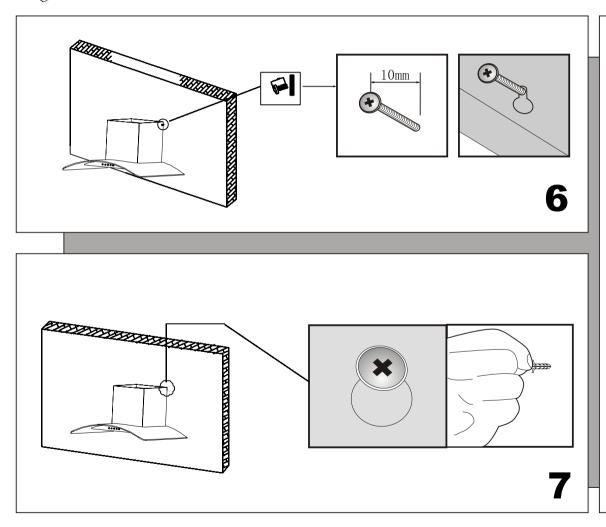
Hang the hood body onto the screws. First screw in the top 2 screws then the bottom 2 screws. Adjust the level of the hood on the wall to be straight horizontally.
