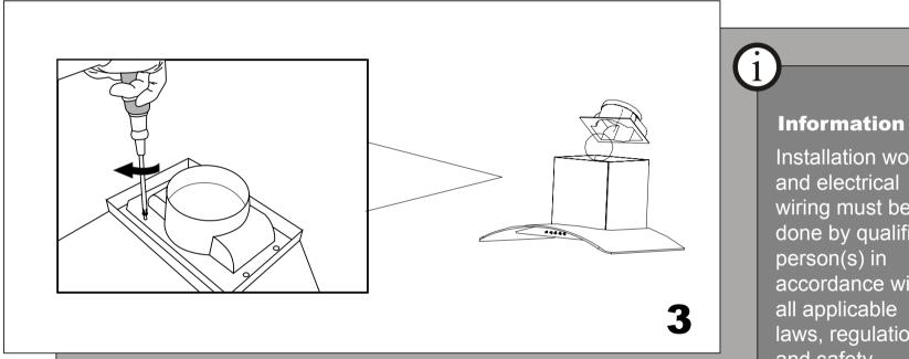
Fig. 3 Attach the damper flap on the air outlet as shown.
