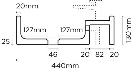
Note: Overflow pipe separate. For surface mount basin, a second hole in bench top is required.
