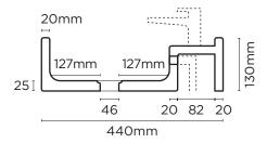
Note: Overflow pipe separate. For surface mount basin, a second hole in bench top is required.
